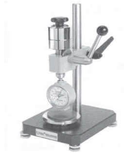
Fig. 4 Hardness Measuring Equipment
