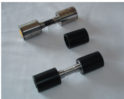
Fig. 39 Corrosion Free Sleeve for Apron Top Roller
