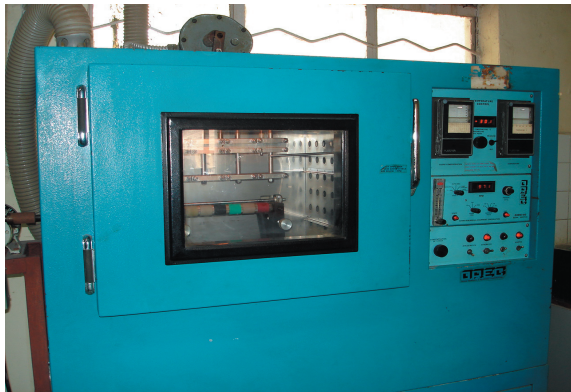
Fig. 30 Ozone Resistance Testing Equipment
